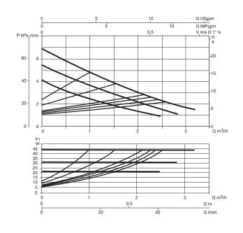
The performance curves are based on kinematic viscosity values = 1 mm $^2$ /s and density equal to 1000 kg/m $^3$ . Curve tolerance according to ISO 9906.
